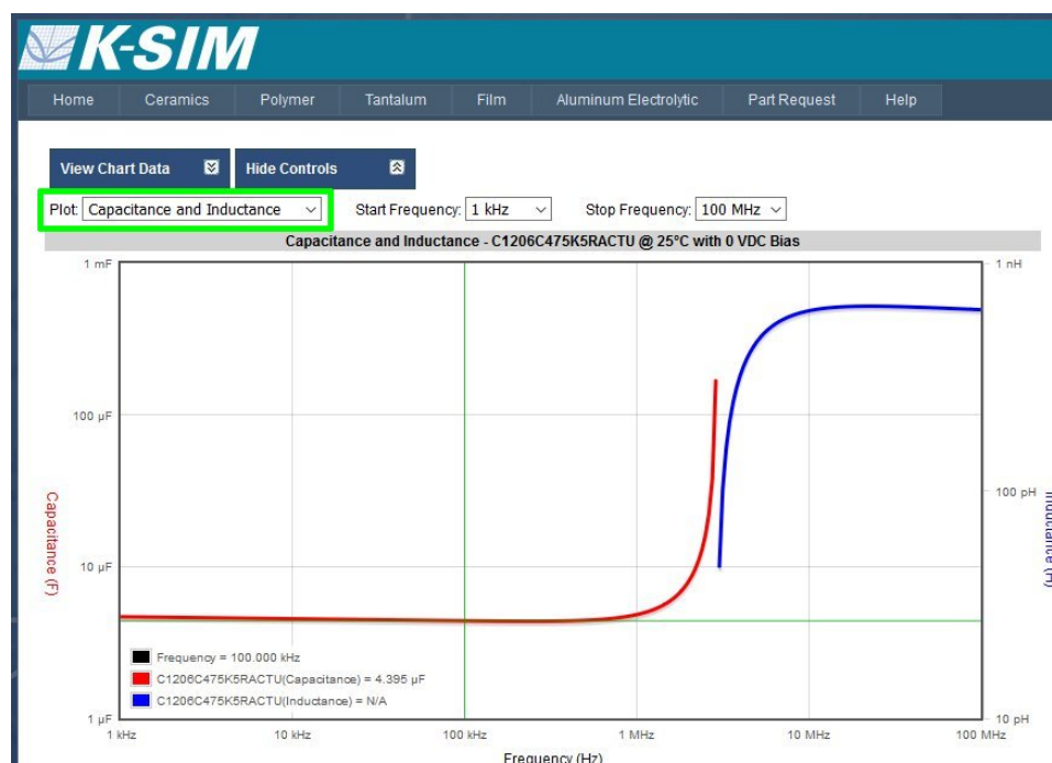
Fig. 6: Manufacturer's design resources tool – actual capacitance as the function of frequency.
