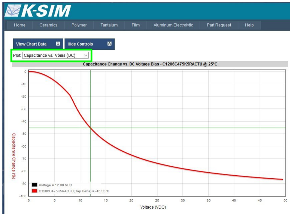
Fig. 7: Manufacturer's design resources tool – actual capacitance de-rating as the function of DC voltage bias.
